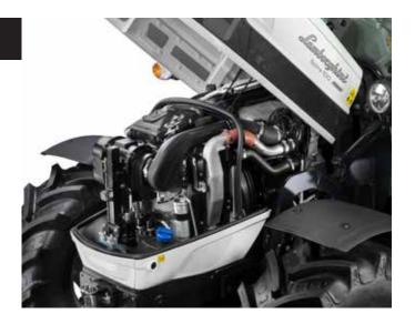
load variations. With the new layout underneath the bonnet, the DOC catalytic converter is positioned in a sheltered, protected area along with the new PowerCore 2-stage air filter (which can be fitted upon request with a dust ejector). To facilitate maintenance, all inspection and service points have been made more easy to access, and the radiator pack is now protected by two practical sliding screens.
